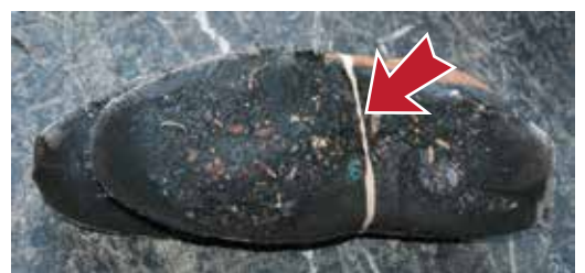
• Soles are melted, distorted and not wearable
